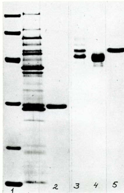
Fig. 1. PAG electrophoresis under denaturation conditions (1-2) and without denaturants (3-5): 1 – protein markers, 2, 3 – nuclease sample after phosphocellulose chromatography, 4 – nuclease S.m. , 5 – nuclease S.m.
